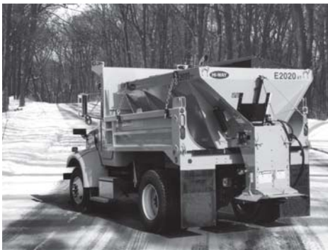
Higher truck speeds will cause the salt from a deicing machine to roll and spread across the road.
