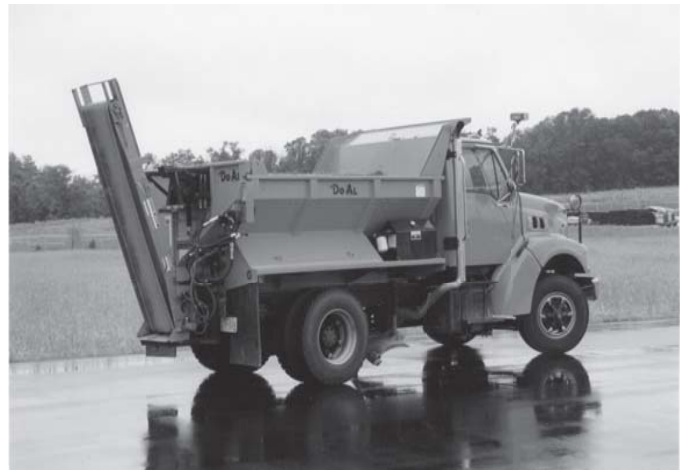
This machine spreads abrasives and chemicals on roads for ice control.
